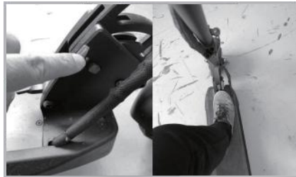
Step6: Unlock the protection pin. Kick down the folding lever and push the handlebar forward to fold the scooter. Always keep protection pin in position when the scooter is unfolded.
